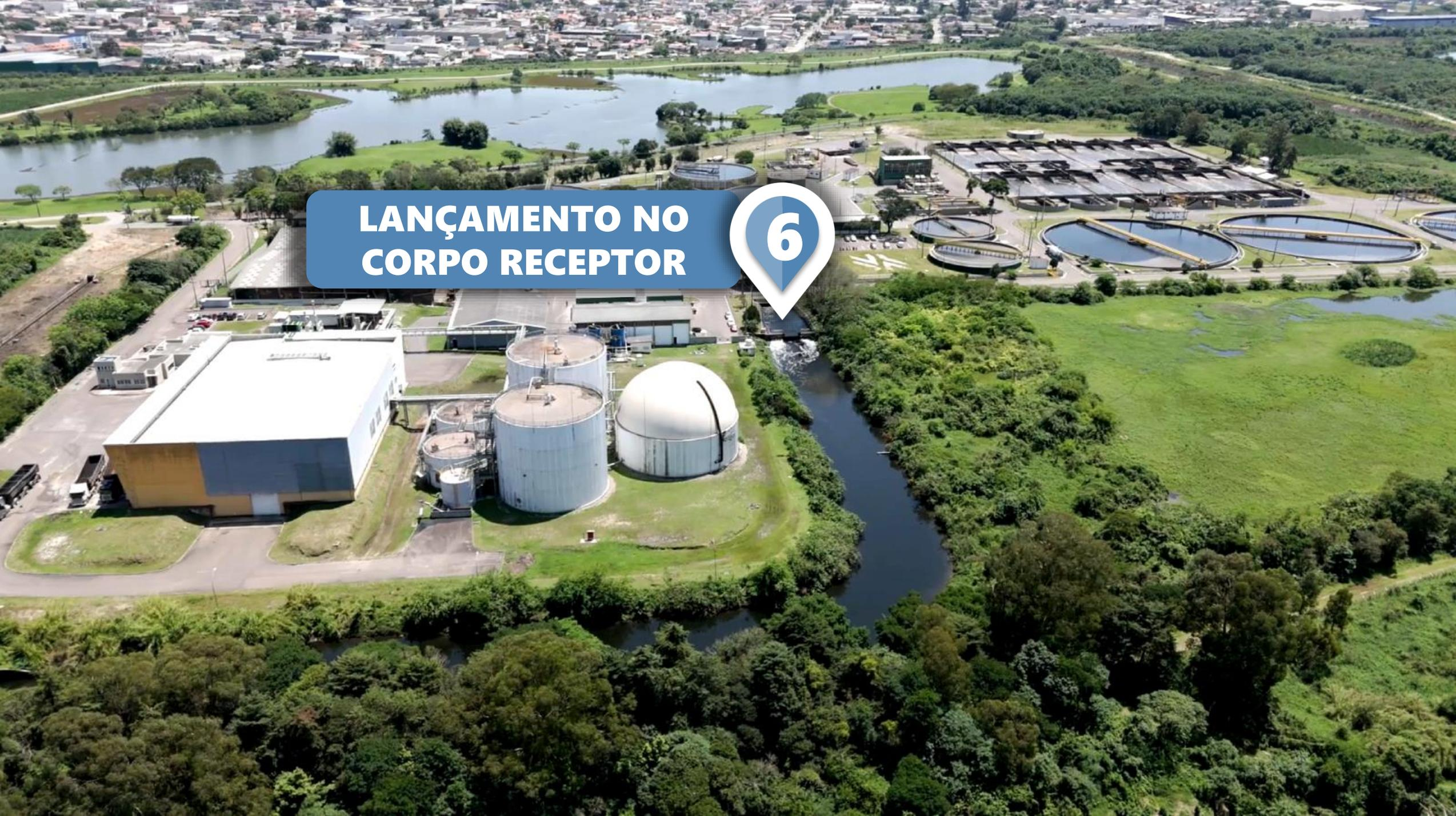
An aerial photograph of a wastewater treatment plant. In the foreground, there are several large, cylindrical tanks and a large white building. A discharge channel flows from the plant towards the right, surrounded by dense green vegetation. In the background, there are several circular aeration basins and a large rectangular building. A city is visible in the far distance.
